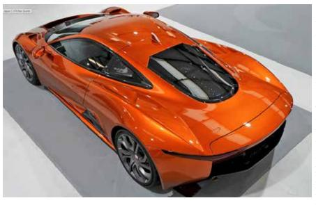
stunt cars were designed to withstand punishing chase scenes. Constructed around a robust, tubular spaceframe chassis with rally-derived suspension and Jaguar's 5.0 litre, supercharged V8 engine, CALLUM's private customer commissioned the Warwick-based team to transform the C-X75 for road use whilst carefully preserving its iconic history. For the complete story, check this out:
