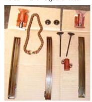
When the worst happens: This 1999 XJ8's tensioners both cracked. When the one at the top left broke, its timing chain (shown) snapped and the valves collided with the pistons. Two of the bent valves are shown in this photo. Though such damage requires significant shop time to repair, engine replacement is usually NOT indicated, and the
